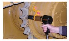
**How Do They Work -** The RAD pneumatic Torque tools are basically an air motor, driving a torque multiplier gear box. The tool will run in forward or reverse at full power by switching the reversing lever similar to an impact wrench. The tool can be pre set to any torque value within its range for torque up, or undo bolting..
