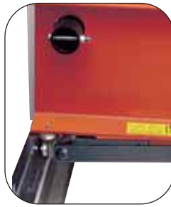
Bearings make bed positioning smooth and easy.
